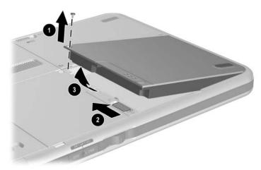
Removing the Battery Pack
